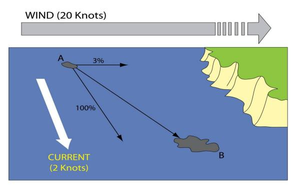
Fig 7: Direction of drift of oil on water - resultant of 100% of the current speed and 3-4% of the wind speed. Source: ITOPF
