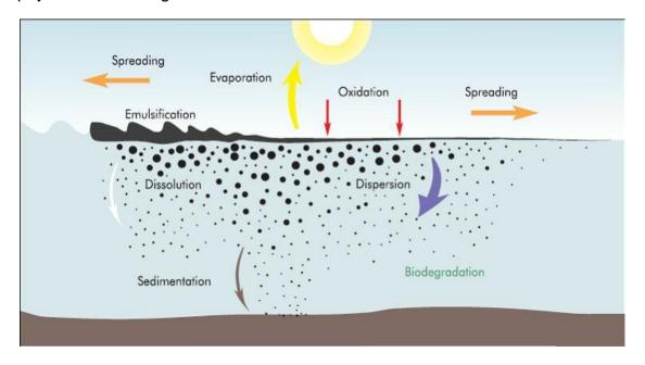
Fig 6: Weathering processes acting on pollutioned oil. Source: ITOPF
