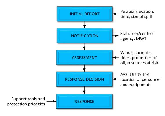
Fig 4: Typical response procedure
