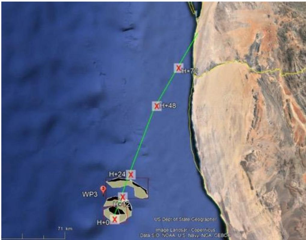
Figure 1: oil trajectory (green line and time markers) according to the MetOcean conditions provided for the exercise and results of aerial surveillance provided to the participants in injects 4, 7 and 9.
