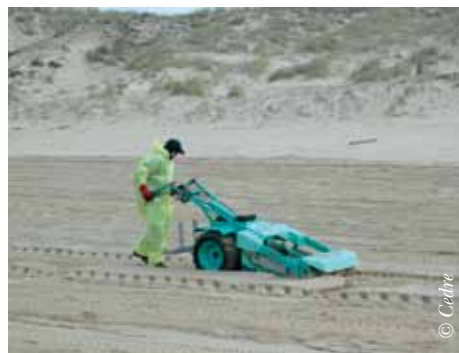
Mechanical selective sand screening
