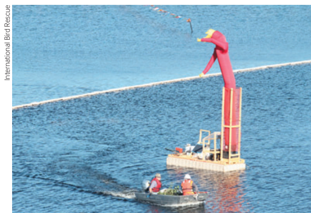
An example of visual hazing equipment deployed from a moored buoy.
