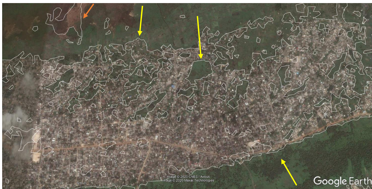
Figure 30: Overlay of urban areas derived from classification method (white line) on high resolution google Earth layer. The map shows good agreement of the urban delineation with the underlying map (yellow arrows) but also wrongly classified urban areas (orange arrow)
