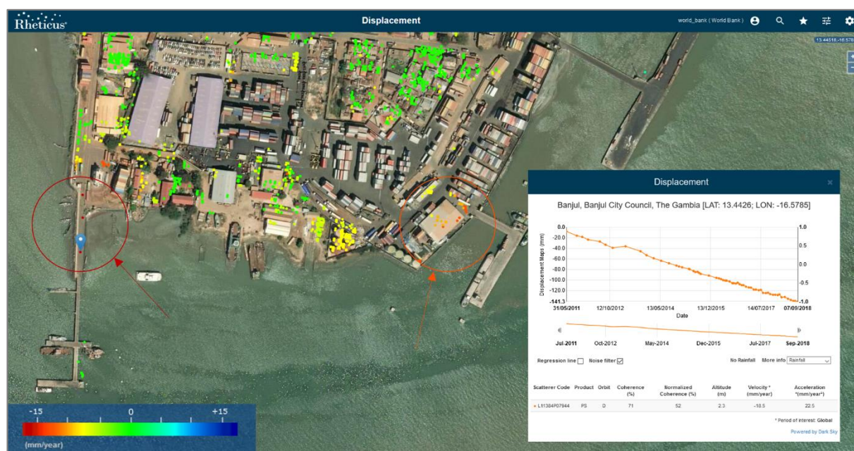
Figure 34: Example of localised ground motion phenomena close to Banjul Harbor, with detailed time series graph of the displacement that shows a total movement of about 14 cm from May '11 to September '18 in the point highlighted in blue. Red and orange circles show clusters with differential terrain movement of more than 10 mm a year
